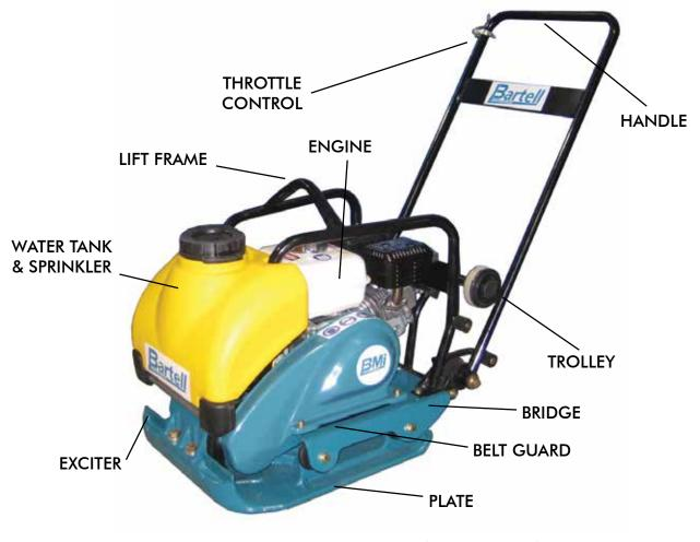
Figure 4: Compactor Major Components (B200 Model Shown)
