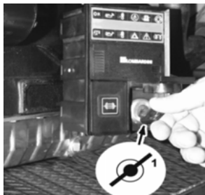
1st position - Warning light on.
