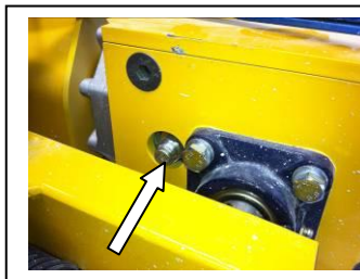
Fig 3 - Oil Level Plug or Level Gauge site
