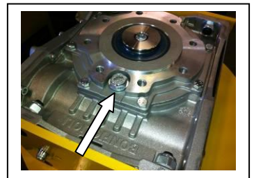
Fig 4 - Gearbox Oil Filler Plug
