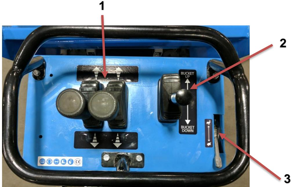
1. **Track Controls:** Forward and reverse controls for each track
