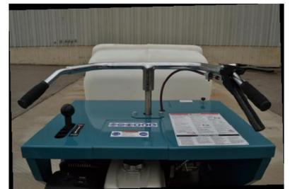
2. **Travel Speed Control** – The travel speed control adjusts the speed at which the buggy travels. Squeeze the handle to increase speed. Release of the handle will stop the machine. The lower handle is forward while the upper is reverse.
