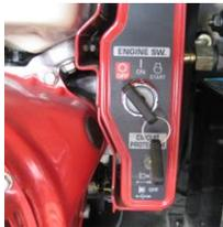
**Electric Start** - The engine control is a three position key switch. The first position (key vertical) is the stop position. The second position is the run position. The third position is the engine start position.
