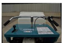
2. **Travel Speed Control** – The travel speed control adjusts the speed at which the buggy travels. Squeeze the handle to increase speed. Release of the handle will stop the machine. The lower handle is forward while the upper is reverse.
