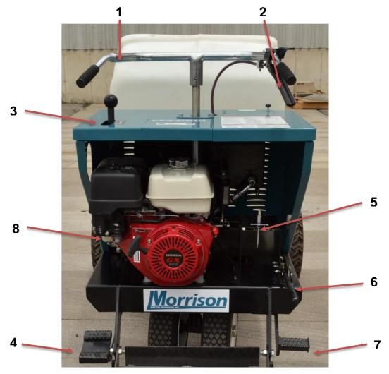
Steering Handle Bar – The steering handlebar is attached to the rear wheels of the unit. Rotating the handle bar clockwise steers the unit to the left. Rotating the handle bar counterclockwise steers the unit to the right.
