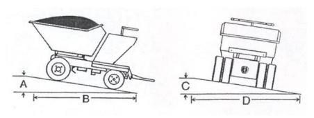
To calculate Grade, divide the vertical rise by the horizontal run and multiply by 100.
