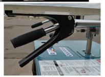
Dump Hand Control – The dump hand control activates the hydraulic dumping mechanism. Push forward to dump bucket. Pull back to return bucket to travel position.
