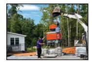
CENTER LIFT POINT Equipped with a Center lift point that allows the iQ1550™ to be lifted into a job site.
