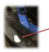
Gear oil fill plug access hole is located on the top of the shroud. Gearbox must be rotated until you see fill plug.
