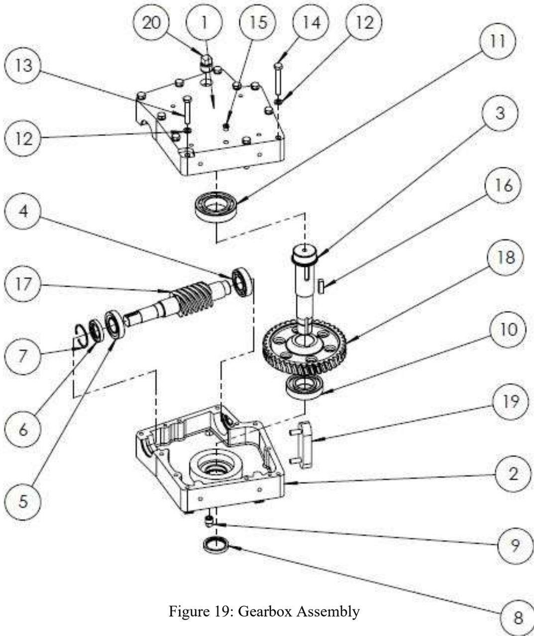
Figure 19: Gearbox Assembly
