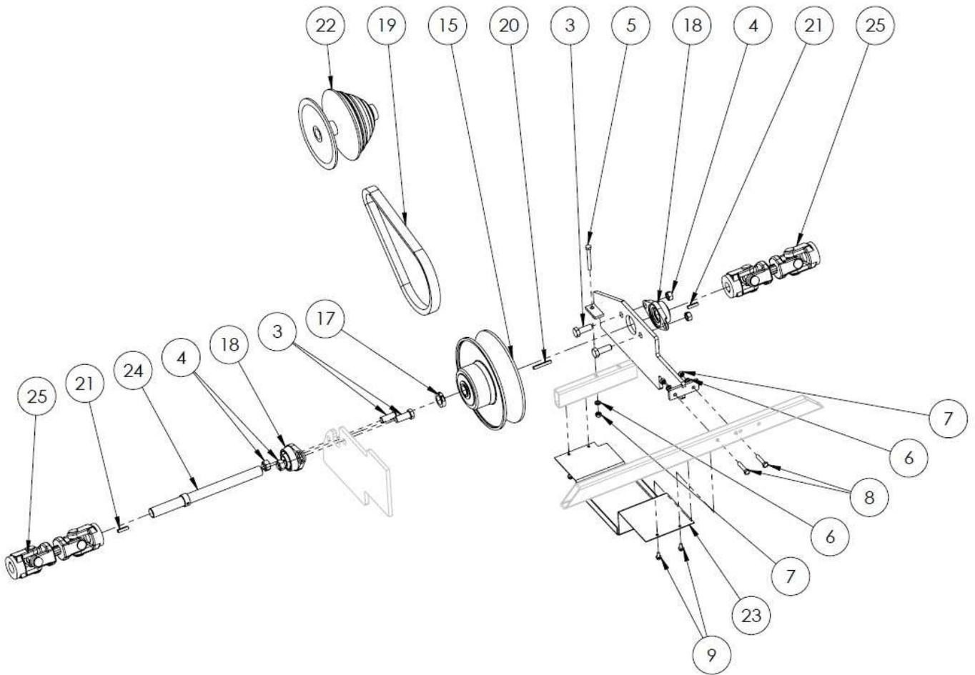
Figure 17: Drivetrain Assembly
