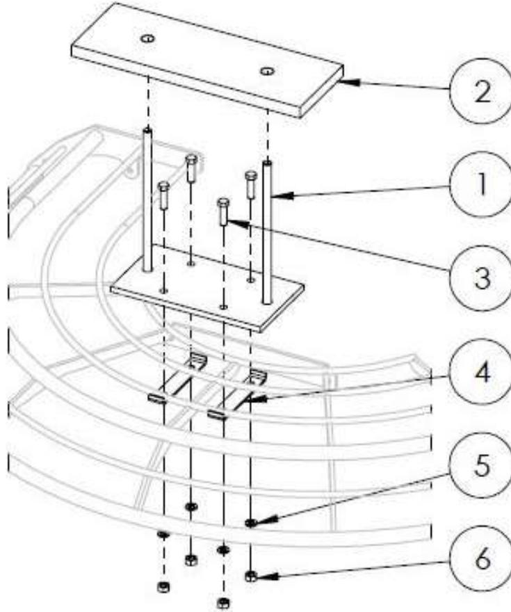
Figure 23: Weight Package Assembly
