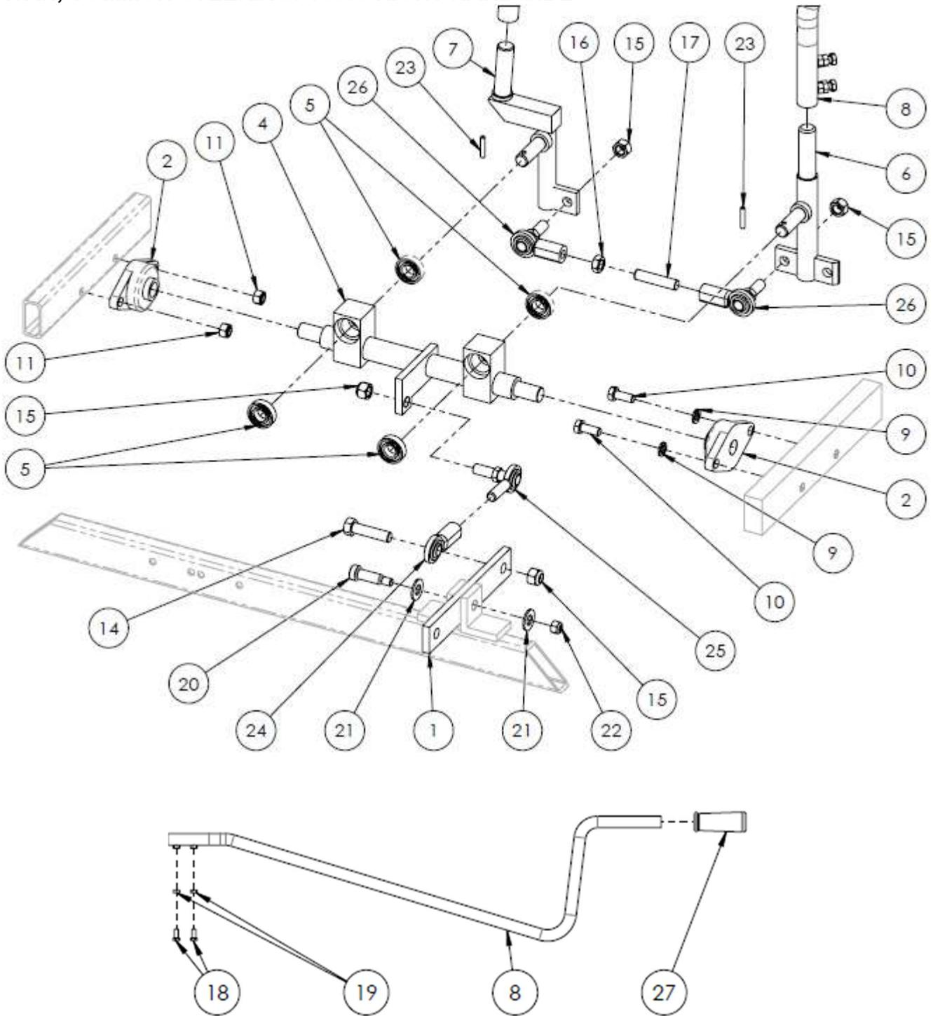
Figure 12: Steering Assembly
