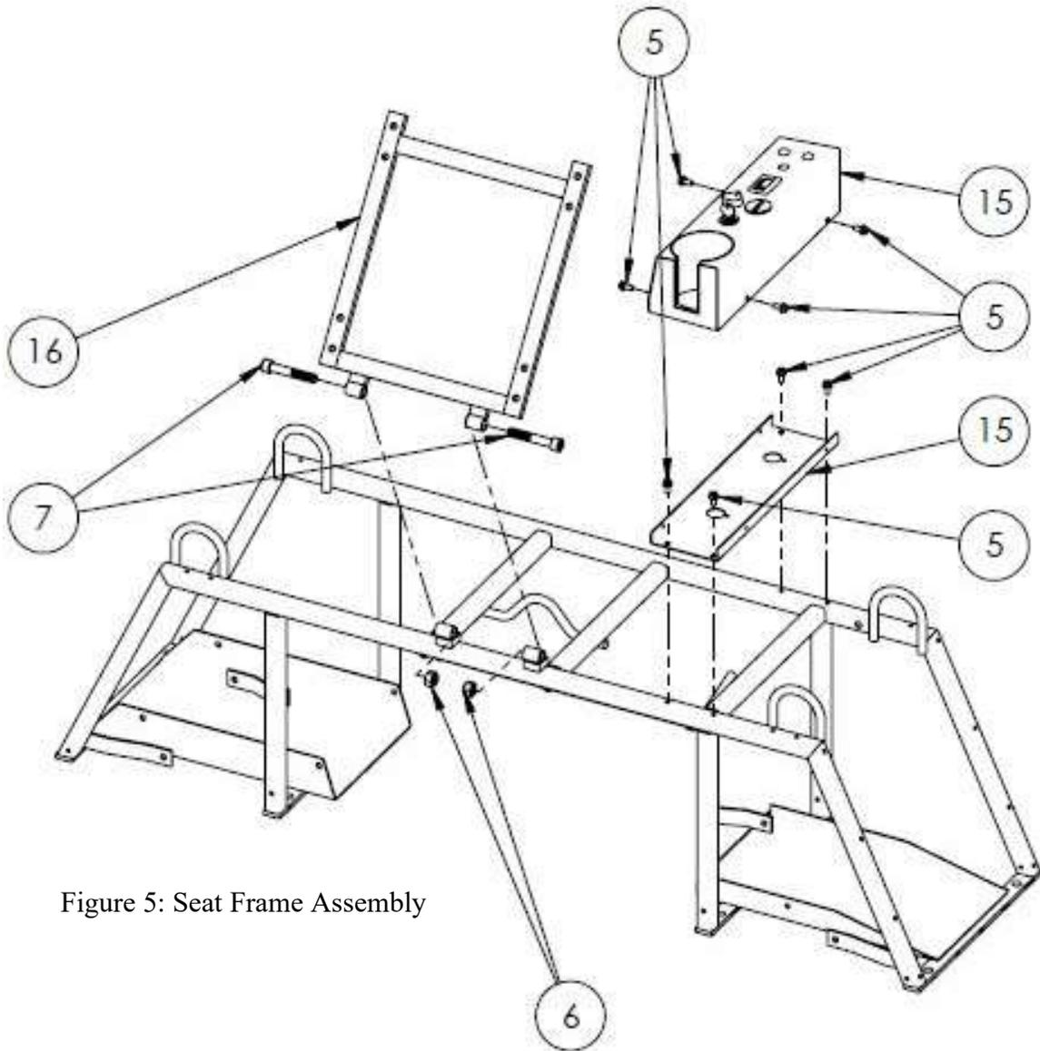
Figure 5: Seat Frame Assembly
