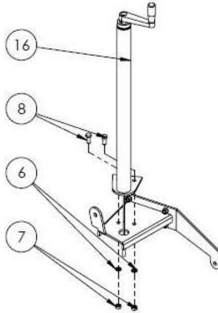
Figure 15: Steering Assembly
