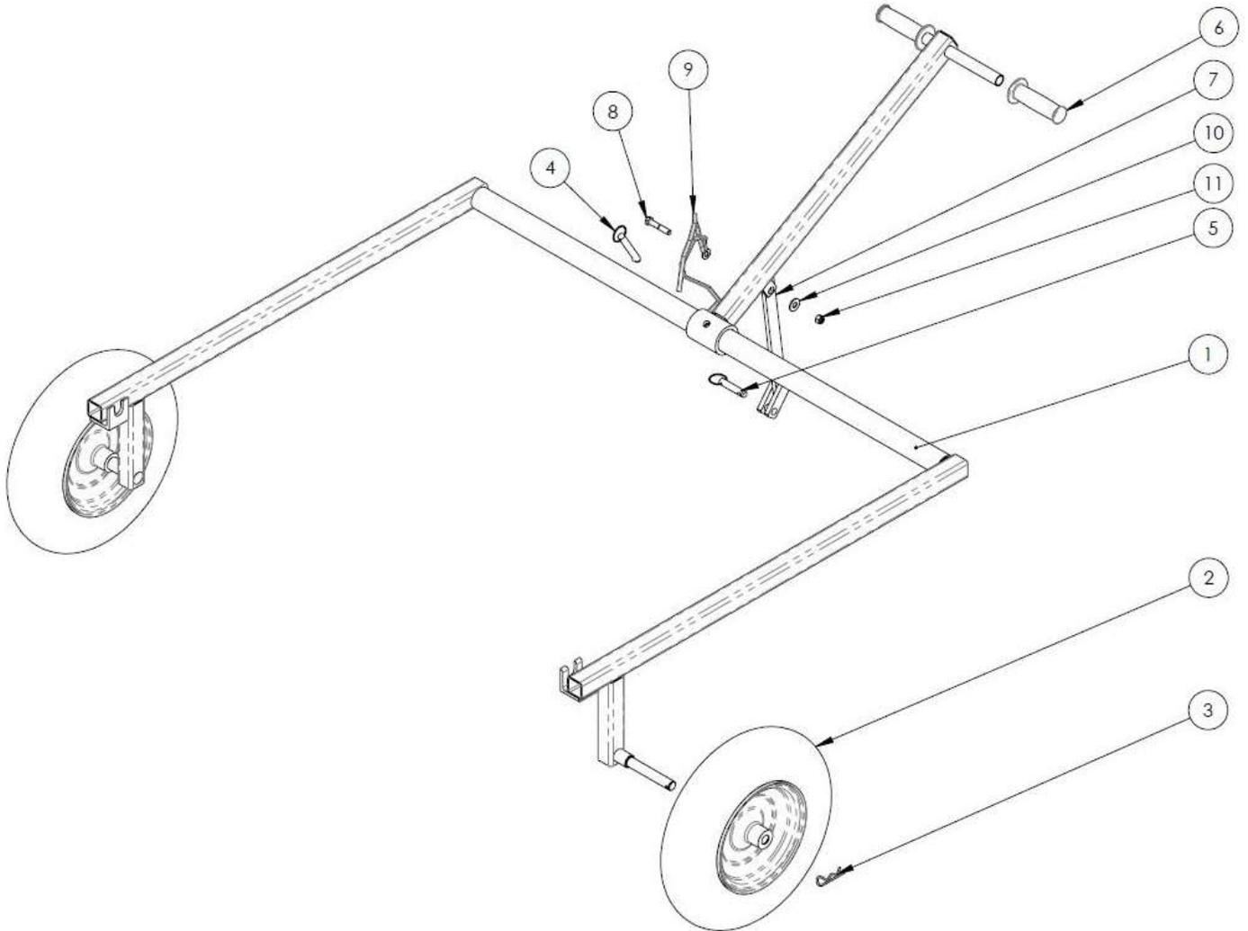
Figure 24: Retardant Sprayer Assembly
