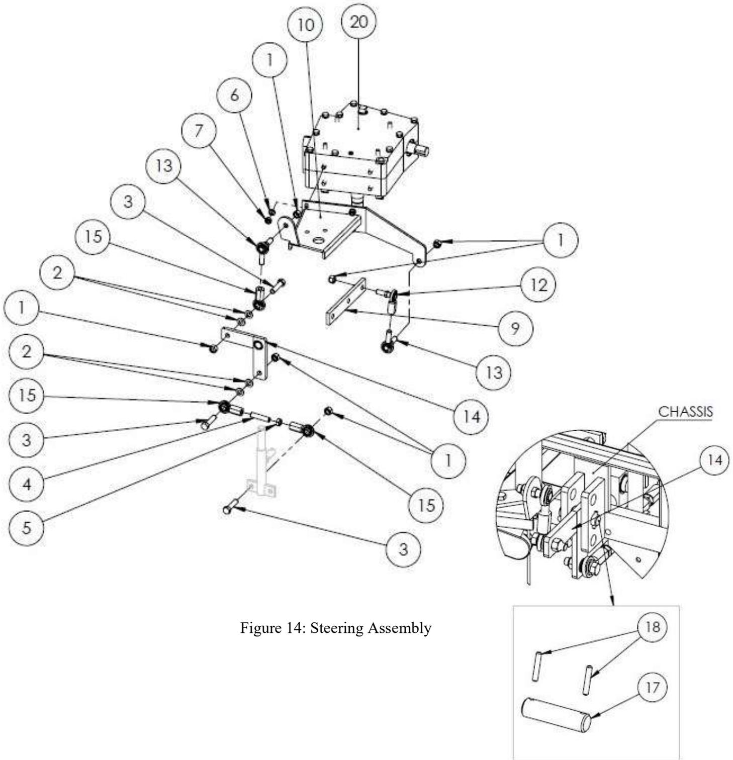
Figure 14: Steering Assembly
