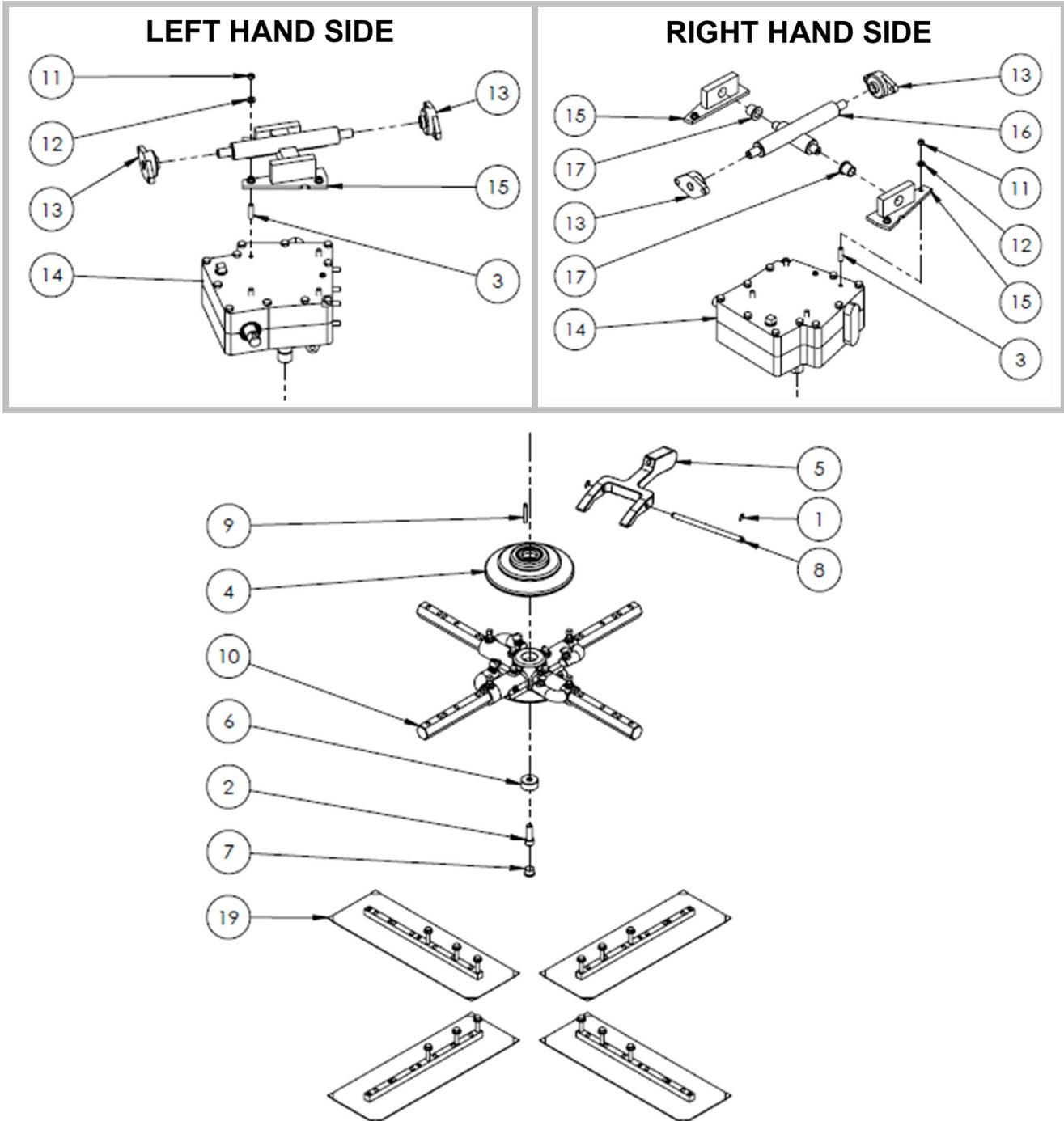
Figure 18: Drivetrain Assembly
